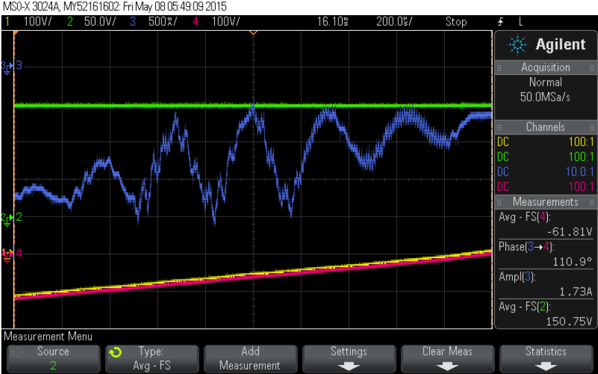
Figure 5-8 ripple current in the unstable zone
