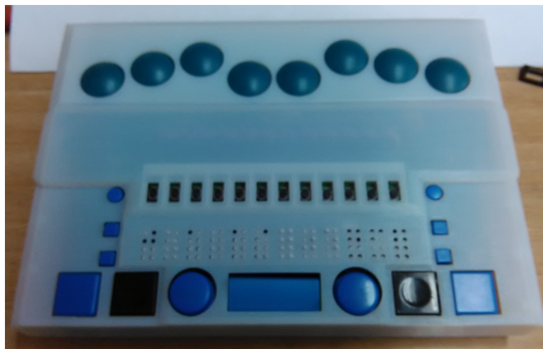
Figure 6.1 Final Braille reader prototype inside it's 3D printed box
