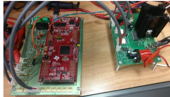
Fig. 14. Cuk converter and digital control printed circuit board.
